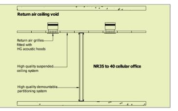
This method utilises HG acoustic hoods, which are detailed in the CAICE Acoustic Hood data sheet. In addition high quality demountable partitioning and suspended ceiling systems are incorporated throughout the office.
