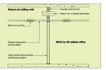
This method utilises acoustic void barriers, penetrated by return air crosstalk attenuators. Although high quality partitioning is still required, a budget ceiling system can be used, as noise between adjacent rooms has to pass through the ceiling and the void barrier.
